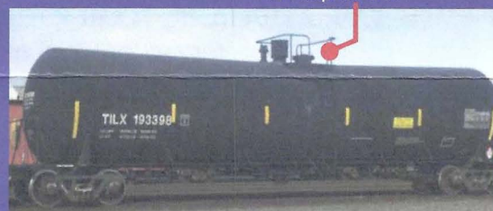
Liquids - Flammable, non haz, food products. Jacketed or non-jacketed.
